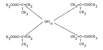
During polymerization the metal clusters tend to weakly agglomerate until solidification eventually traps them. The metal is apparently incorporated in the polymers and can be detected by high resolution mass spectrometry, CIMS.
